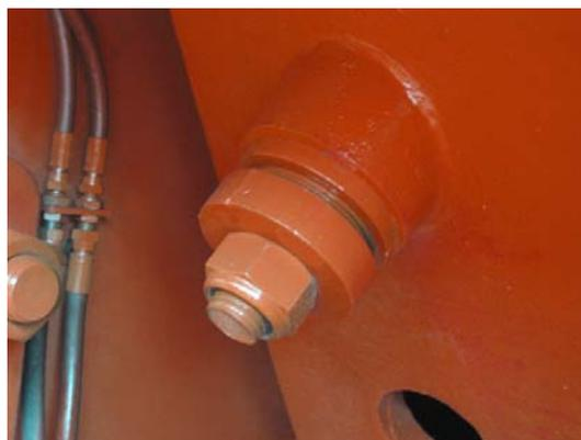
12. Remove the wedge bolts and the wedges from swing jaw stock only.
