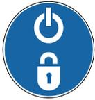
In the event of material blockage, any malfunction or operational difficulty, stop equipment and lockout immediately. Rectify problem immediately, Refer to *Stalled or Blocked Crusher*, page 122 section or contact your nearest dealer.
