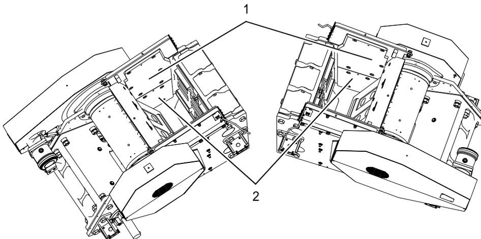
**Figure 6-7: Location of crusher box liner plates**
