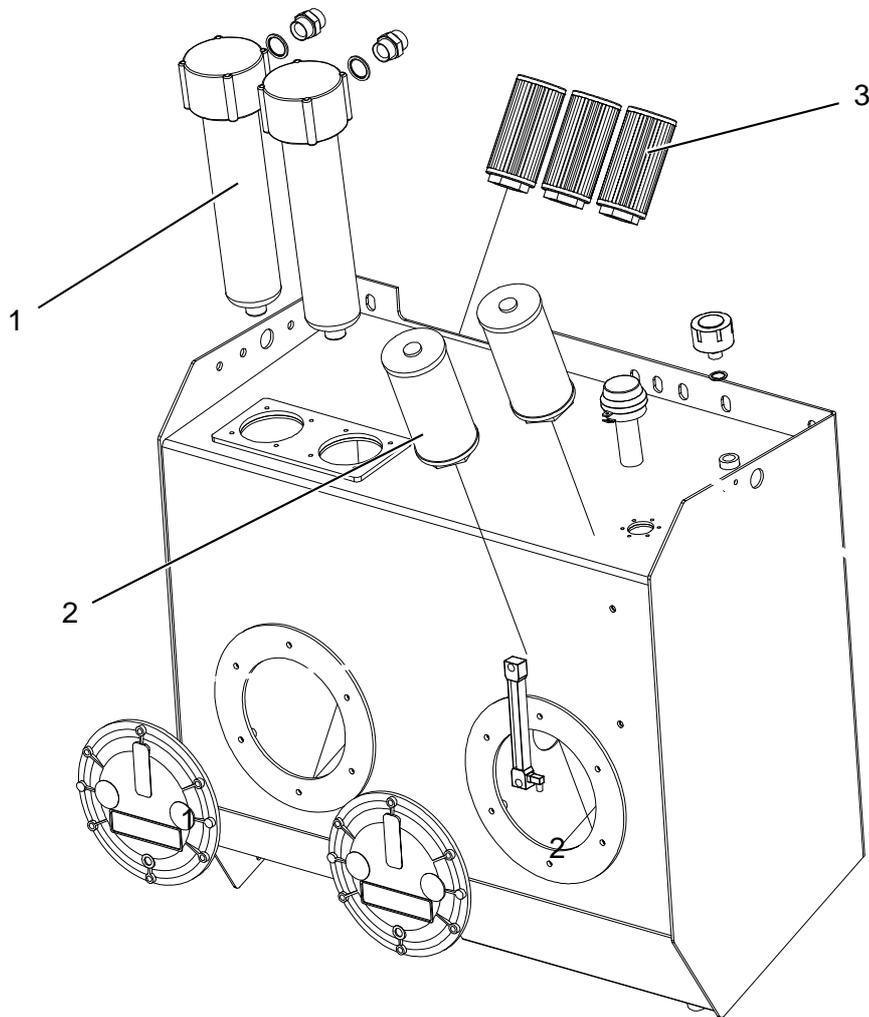
**Figure 6-5: Hydraulic tank - filter element locations (for replacement)**
