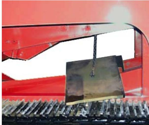
11. Check and Inspect the Toggle clamp and toggle ram bearings for cracks. Replace if necessary.
