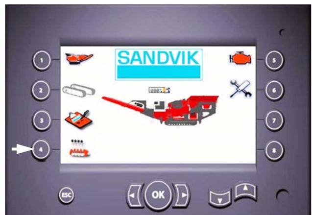
**Note:** *The purpose of lowering the jacking legs is to support the vehicle weight and distribute the load evenly. Some adjustments may be required depending on the site area.*
