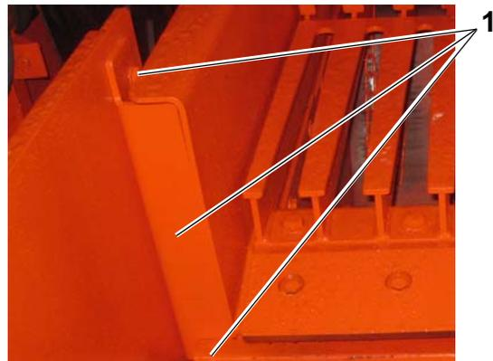
2. Place the lifting tools in the jaw plate. Before lifting the plate make sure the back face and pockets are clean of debris.
