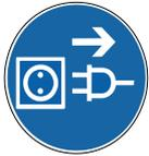
Before starting any maintenance or repair work, the power supply to the equipment **MUST** be isolated. Check the de-energized parts to ensure they do not have any power. In addition to insulating any adjacent parts or elements, ground or short circuit them to avoid the risk of electrical shock.
