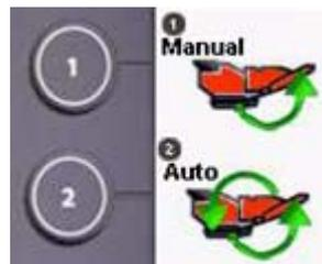
The procedure may be repeated as often as necessary to try to release any blockages in the crusher box. If the machine is unable to crush material that has become stuck in the jaw after the crusher reverse function has been activated, the crusher may need to be cleared manually refer to **Stalled or Blocked Crusher, page 122**.
