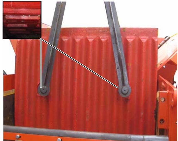
12. The hydraulic ram release with the fixed jaw plate removed, looks as shown.
