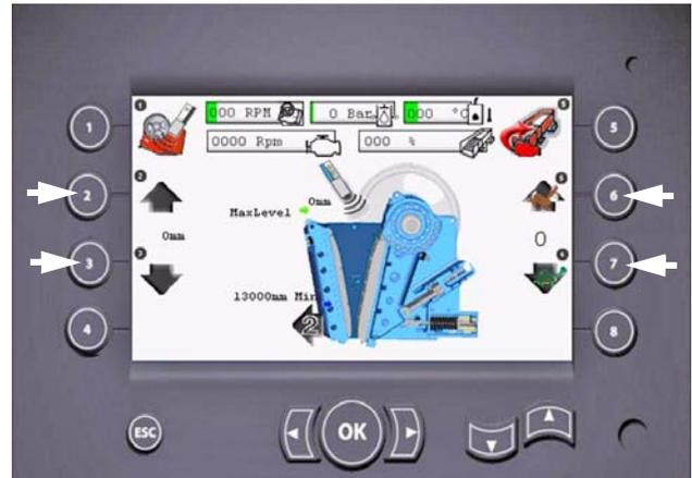
Figure 4-9: Hopper Level Control - Sub Menu
