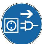
To avoid the risk of electric shock, **ALWAYS** isolate this equipment from the supply source before removing any guards or covers or performing any maintenance or adjustment to the equipment.
