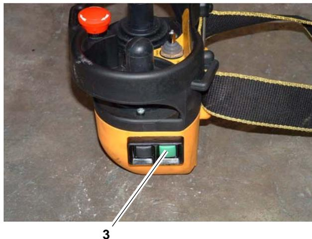
8. If necessary engine Revs Per Minute (RPM) can be adjusted up (faster) or down (slower) to aid tracking using buttons as shown.
