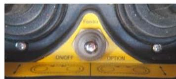
4. Switch the radio remote control to 1 and wait until the green light flashes consistently.
