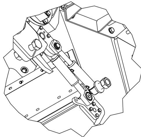
12. Use a minimum of a 2 tonne crane to lift and hold the Toggle plate into the correct position.
