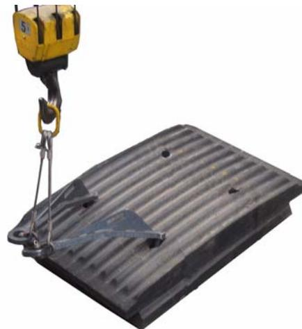
3. Make sure the lifting tool is installed correctly in the hole. Lift the fixed jaw plate with a minimum of a 5 tonne (Metric) or 6 ton (US) crane.
