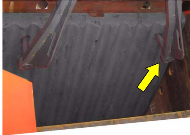
7. This is WRONG. The swing jaw must have no clearance with the jaw face. Adjust the swing jaw plate with the crane.
