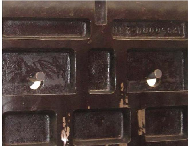
4. Make sure the back of the plate is clean and smooth. Clean out any build up dirt or dust in the holes.
