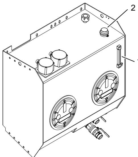
6.10.6. Engine Coolant - Check Level and Top Up
