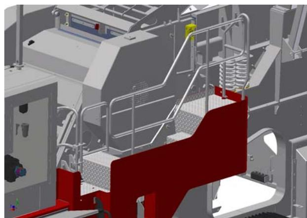
14. Lower hopper lid, install and tighten two bolts (1) each side.
