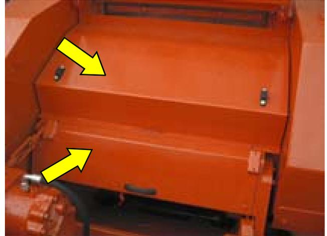
2. Install the inlet chute cover (1).
