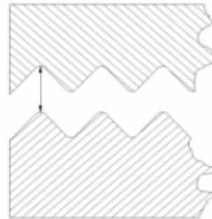
1. On the display screen, from the manual/auto run select screen. Select the right arrow to close the jaw and reduce the CSS.
