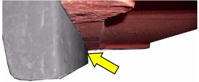
9. Carefully remove the lifting tools, and hold the plate into position, DO NOT ENTER THE JAW BOX.
