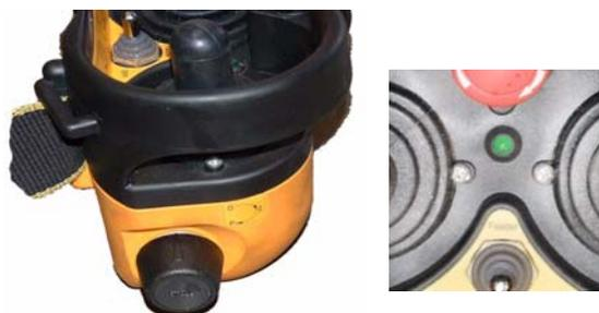
5. Synchronise the radio control to the machine, press green button.
