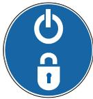
When carrying out any maintenance or working on or around the machine it must be switched off, the isolator moved to the off position and a lock attached to prevent any accidental attempts to start the machine.
