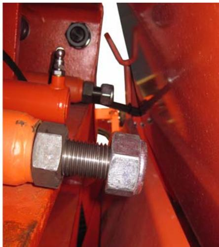
12. Adjust the fixed jaw plate as necessary and make sure it is centred.
