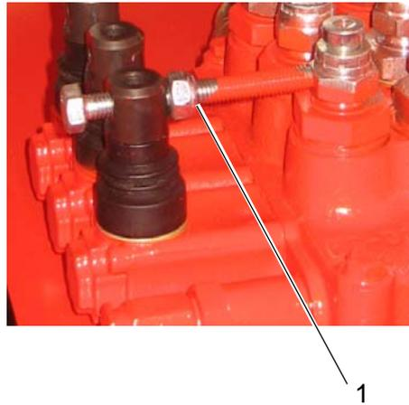
18. Remove the chain and loosen and remove the lifting eye.
