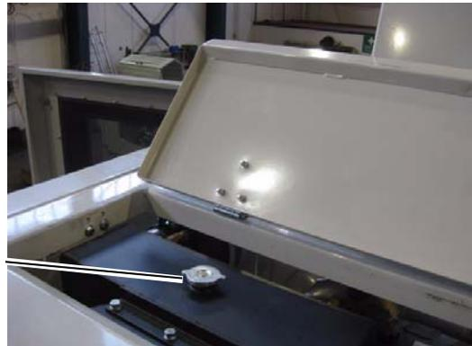
6.10.7. Checking/ Changing Hydraulic Tank Air Breather
