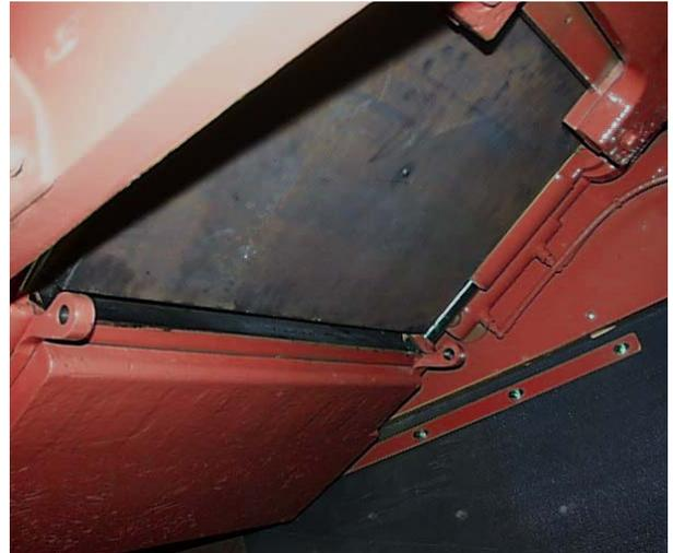
13. Install the tie bar. Install and tighten the bolts with the washers and bushes. Do both tie bars.
