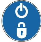
Switch off and lockout equipment before removing any safety devices or guarding. Ensure safety devices and guards are all installed correctly before lock out is removed.
