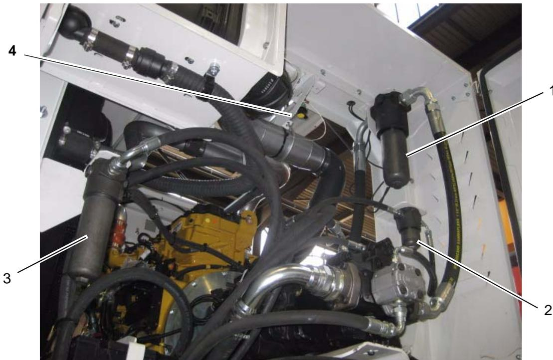
Figure 6-4: Engine Compartment - Filter element locations (for replacement)
