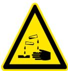
The battery contains sulphuric acid, an electrolyte which can cause severe burns and produce explosive gases.
