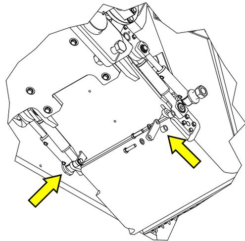
6. Loosen and remove the nut with the bolt. and install and tighten the spare lever onto the toggle plate removal valve (1).
