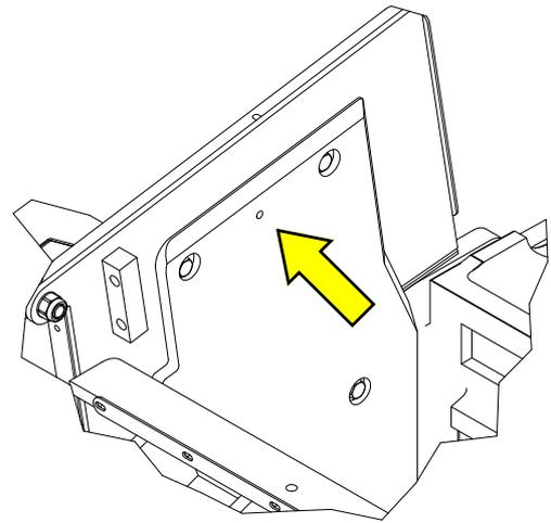
4. Loosen and remove the bolts with the washers. Lift up the wear plate with the crane. To install lift the wear plate into position and hold it there with the crane. Install and tighten the bolts with the washers and nuts (TORQUE 711 Nm).
