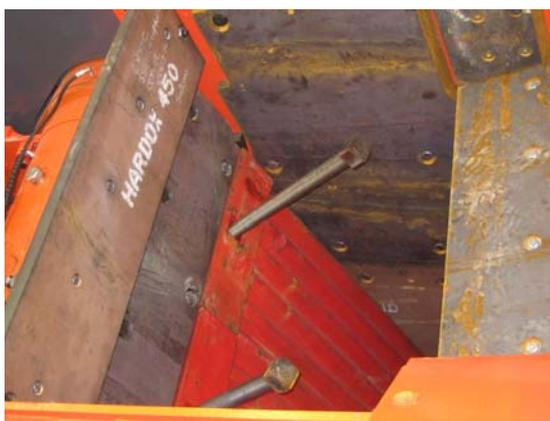
14. Attach a crane to the wear plate and support the weight with the chain/strap. Remove the nuts and the bolts. Remove the wear plate with a crane.
