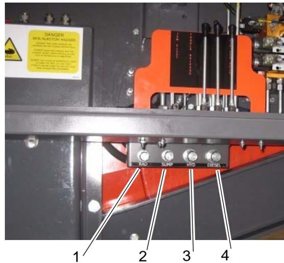
Figure 6-2: Fluid drain points
