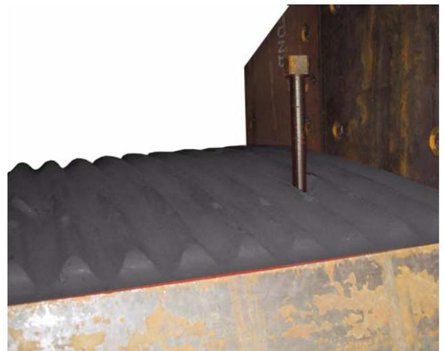
11. Install the nuts and lock nuts, but do not tighten.
