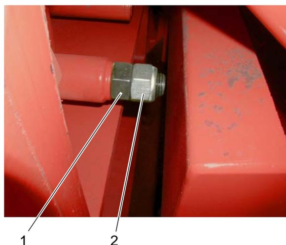
14. Put the sealing plates (both sides) in the correct position against the fixed jaw plate. Install and tighten the bolts (1).
