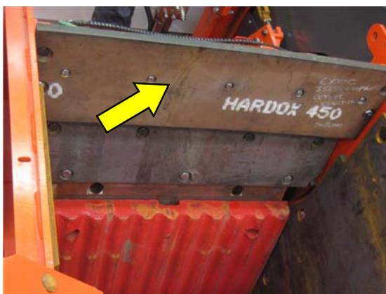
15. Attach the lifting hooks to a minimum of a 5 tonne (metric) or 6 ton (US) crane.
