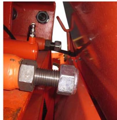
2. Carefully remove the bolts. **DO NOT** enter the crusher box. **NOTE:** Push the bolt from back of the fixed jaw plate.
