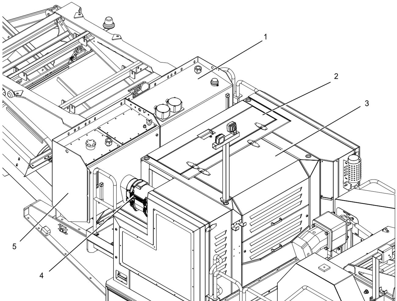
**Figure 6-1: Engine/hydraulic compartment locations**
