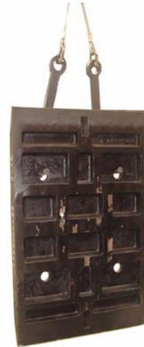
5. Install wedge in position as shown. The wedge should not rest on the lifting tool. See photos for approximate position. NOTE: Use grease to hold the wedge into position.
