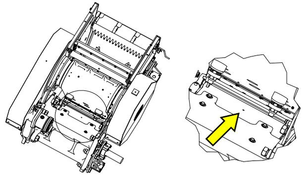
5. Loosen and remove the bolts with the washers and bushes. Remove the tie bar. Do both tie bars.
